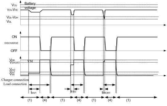
Figure 5-2 Overdischarge Current Detection
