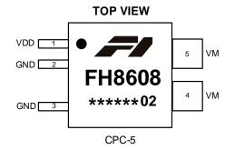
Figure 2. Pin Configuration (Not to scale, \* there are changes)
